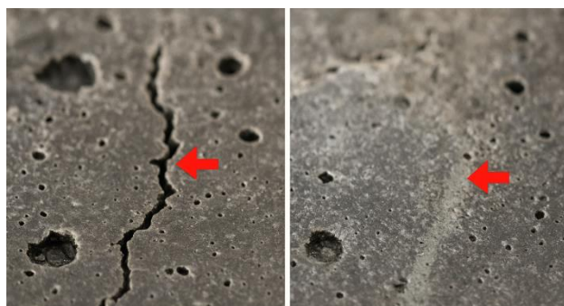
Crack-healing activity in mortar by sodium alginate microencapsulated bacterial spores formed by freeze drying
