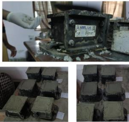
Figure 3 Moulding of Concrete
