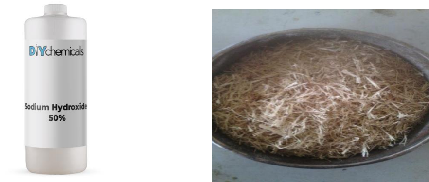
Fig.3. Teat-containing sugarcane in sodium hydroxide solution
